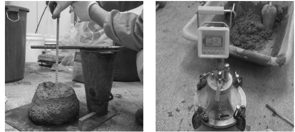
Fig. 2. Slump and air contents test
