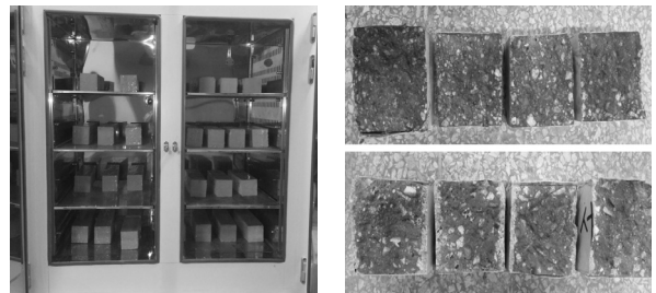
Fig. 4. Accelerated carbonation test
