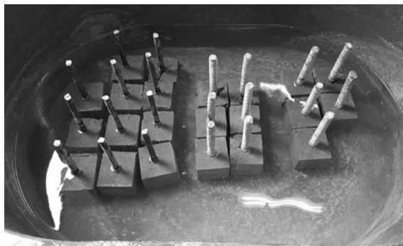
(b) Concrete samples under curing
