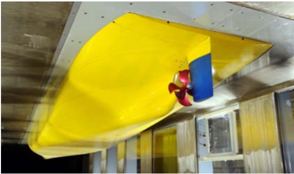
Fig. 7 Model ship installed in LCT test section
