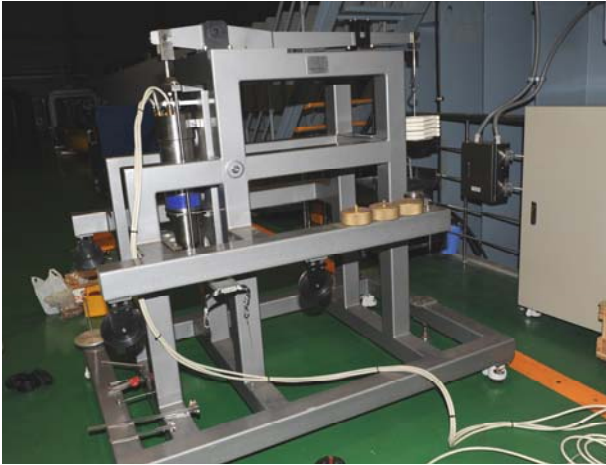
Fig. 3 Calibration for CRP Dynamometer
