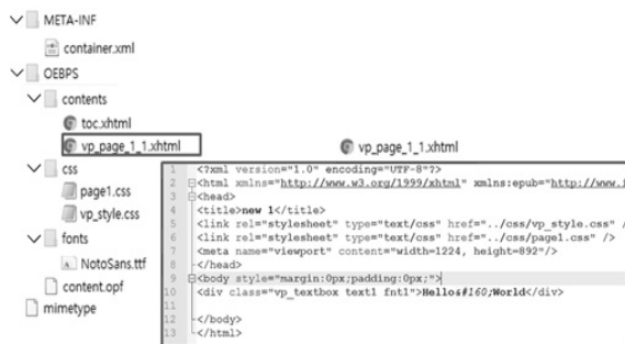
Fig. 4. 'Hello World' Representation Structure in EPUB 3.0
