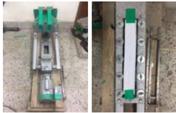
Fig. 9 Small Wheel Track Tester for Adhesion Test
