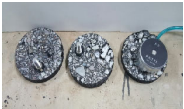
Fig. 6 Mounted Pull-out Stub on Asphalt Specimen
