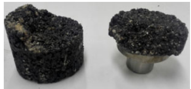
(b) Failure of Upper Level Specimen
