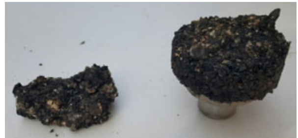
(a) Failure of Lower Level Specimen
