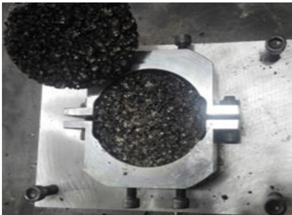
(b) Debonding Shape of Specimen
