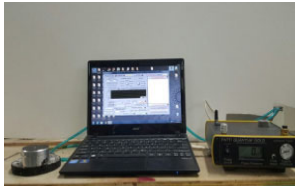
Fig. 5 PATTI Test Set Up
