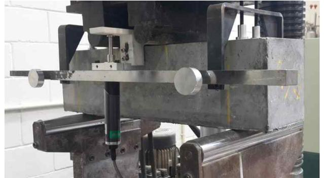
Figure 1. Testing setup for flexural strength and toughness of SI-HPFRCC
