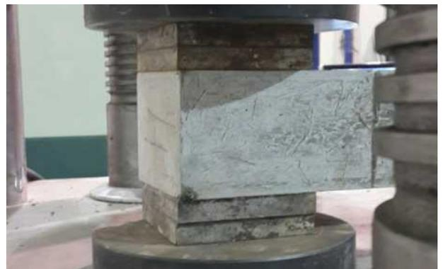
Figure 2. Testing setup for compressive strength and toughness of SI-HPFRCC
