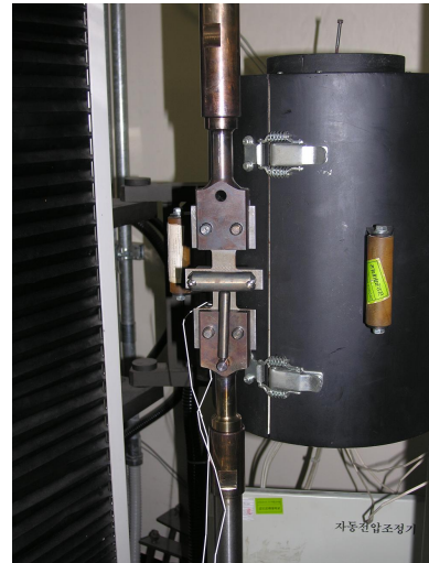
Fig. 8 Test setup for formability with high temperature tensile tester
