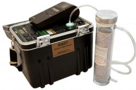
Fig. 1 RAD7 radon measuring instrument was used for measurement of indoor radon concentrations.
