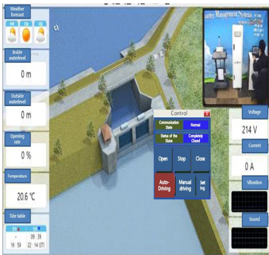
Fig. 7 Controlled water level setting screen
