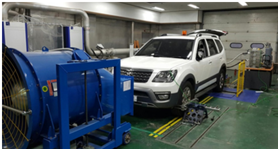
Fig. 3 Photograph of diesel vehicle installed on chassis dynamometer
