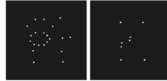
Fig. 5. The corner points of the letter(한, K) by the Harris corner detector
