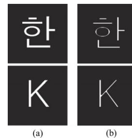
Fig. 3. Before (a) and after (b) the erode operation was carried out.
