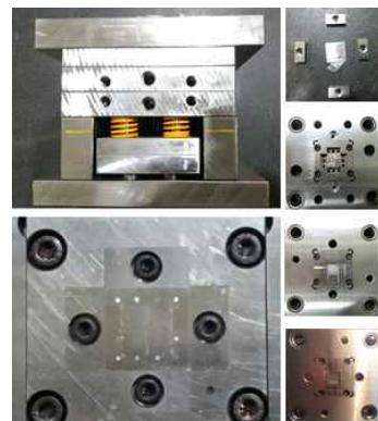
Fig. 4 Standard Mold and important parts
