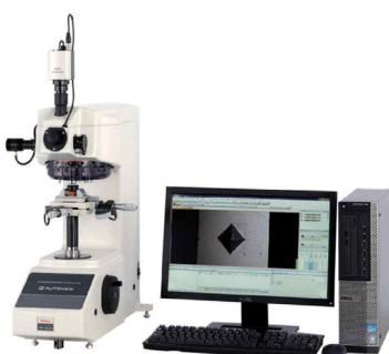
Fig. 2 Automatic micro hardness tester
