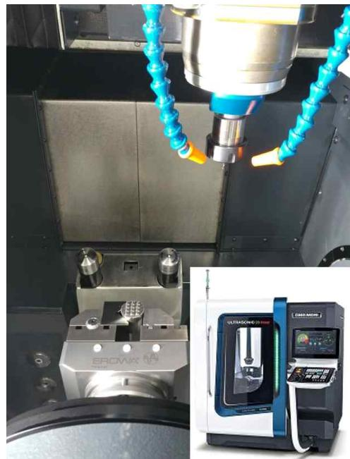
Fig. 9 CNC milling machining center
