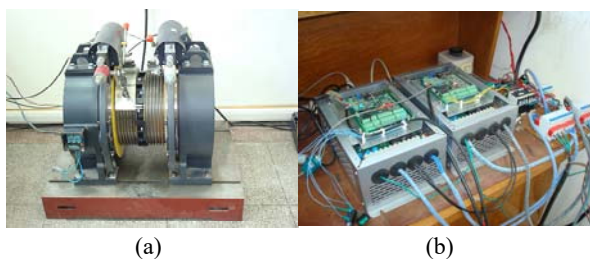
Fig. 9. Experimental platform of 11.7kW elevator traction machine. (a)Traction machines. (b) Drives.
