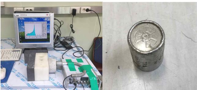
Figure 2. Experimental setup for neutron shielding performance test
