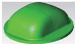
Fig. 1. 3D model of optimized lens for rectangular target.
