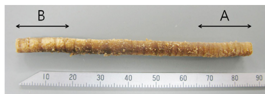
Figure 2. Sample for analysis of FT-IR, solid state ^{13}\text{C} NMR, XRD. (A) Outer part, (B) Inner part.
