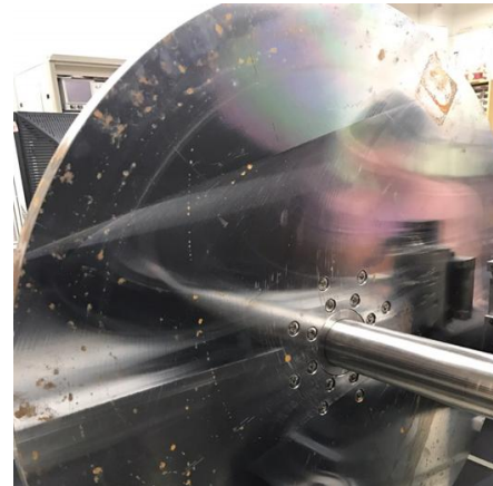
Fig. 12 Solid type mock-up disk brake specimen
