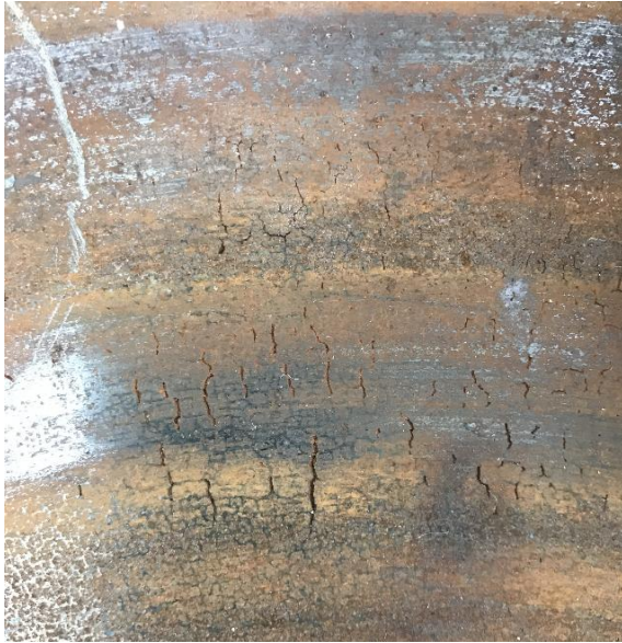
Fig. 1 Photo of surface cracks on KTX disk brake
