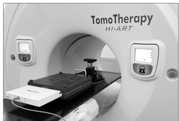
Fig. 3. Phantom setup image for the dose measurement in the Tomotherapy.
