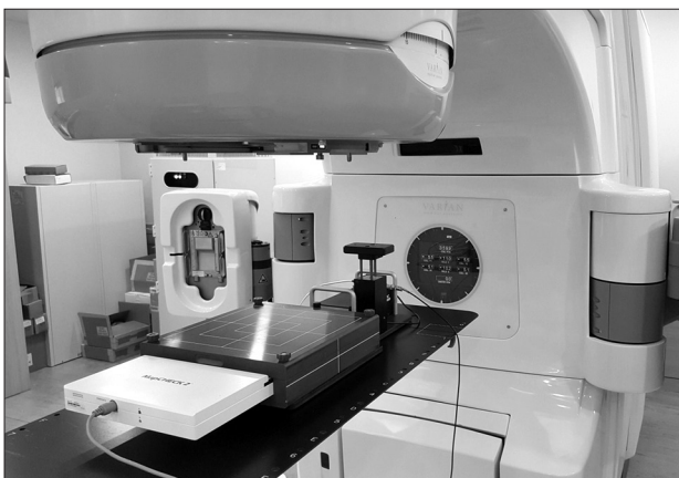
Fig. 2. Phantom setup image for the dose measurement in the Novalis Tx.
