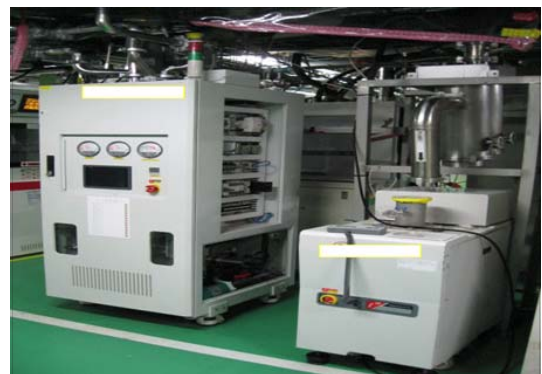
Fig. 3. Primary Scrubber(Left) and Incident Vacuum Pump(Right).
