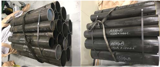
Fig. 1. Testing material-ASTM 106, 53 Gr.B.
