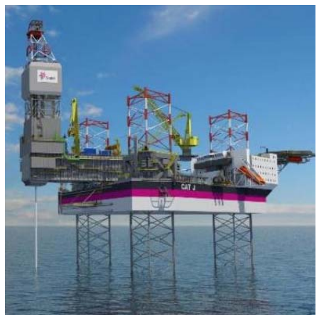
Fig. 1 A typical jack-up drilling unit
