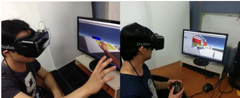
Figure 7. Controlling the 3D virtual environment with Oculus Rift and Leap Motion (left) and controlling the 3D virtual environment with Oculus Rift and Xbox controller (right) during the Iteration 1
