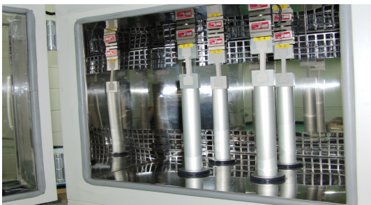
Fig. 5 Verification Test of Endurance Tester.
