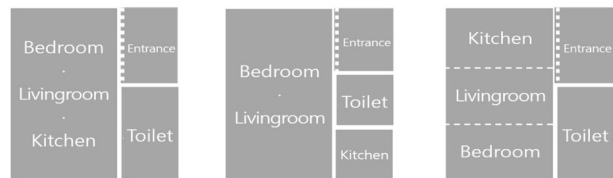
Figure 1. Space Construction of One-room Studios
