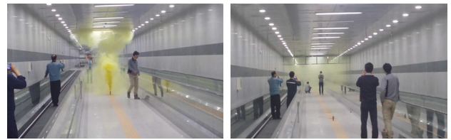
Figure 15. C zone fire causes smoke to spread from C zone to B zone (1st test).
