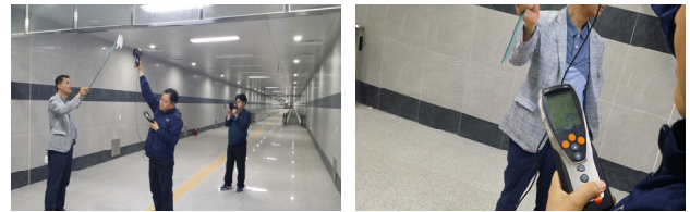
Figure 16. The measurement of natural wind and train wind in underground transit passage.
