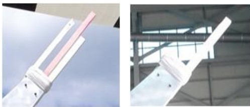
Fig. 9. Safety stick configuration after ground taxi test[2]
