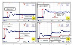
**Fig. 5.** Magnetic bar's angle of Arago's disc controlled at 45<sup>0</sup>(a), 90<sup>0</sup>(b), 120<sup>0</sup>(c), and change controllers with time(d).
