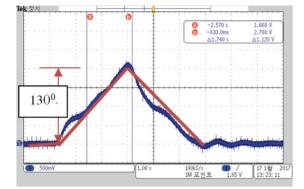
Fig. 8. Waveform output at a change controller with reference angle range in increment/decrement.
