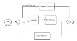
Fig. 1. Schematic diagram of gain scheduling control system.
