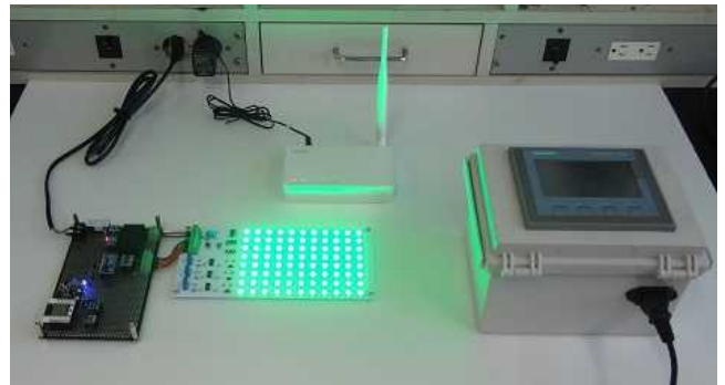
Fig. 9 Implementation of modbus TCP LED control system
