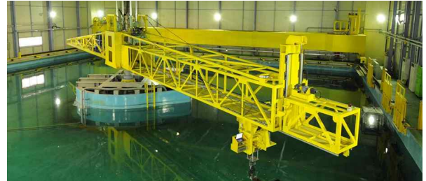
Fig. 2 Photograph of the rotating arm facility
