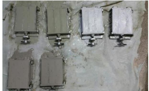
Fig. 3. Depositing pile-filling materials in mold
