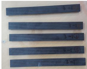
(b) ASTM D790 flexure test specimen
