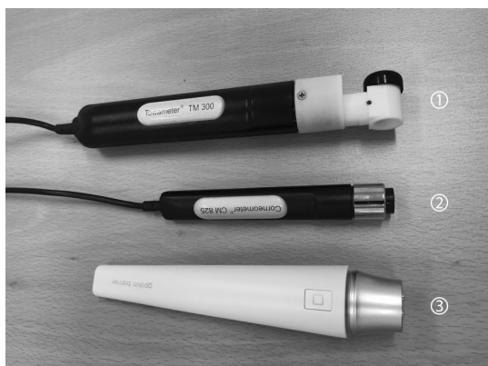
Fig. 2. The Measurement Equipment ①Tewameter® TM-300 (Courage-Khazaka Electronic, Germany), ②Corneometer® CM-825(Courage-Khazaka Electronic, Germany), ③ Gpskin barrier®(G power, Korea)
