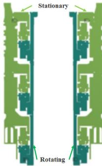
Fig. 4 Cross section of shaft seal
