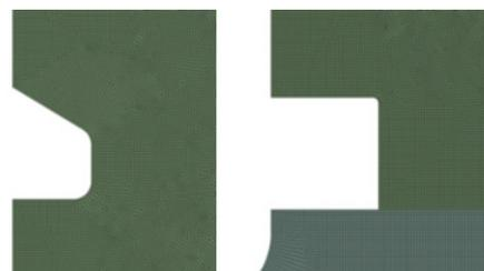
Fig. 5 FE model for shaft seal
