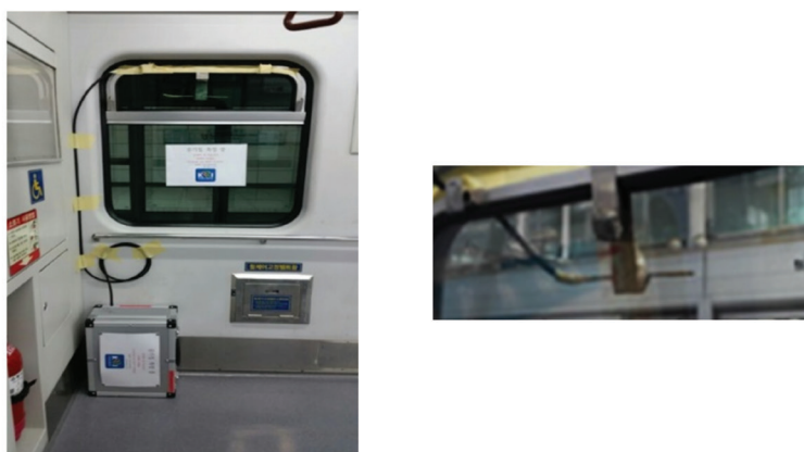
Fig. 1. Photos for a sampling location and an inlet tube in a subway passenger cabin.
