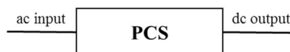
Fig. 4. Converter mode of the PCS for evaluating the AC to DC power conversion efficiency.
