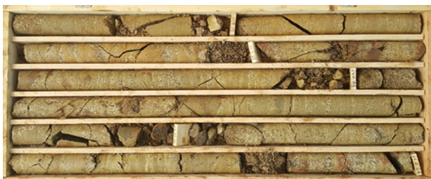
Fig. 2. Weathered rock core sample
