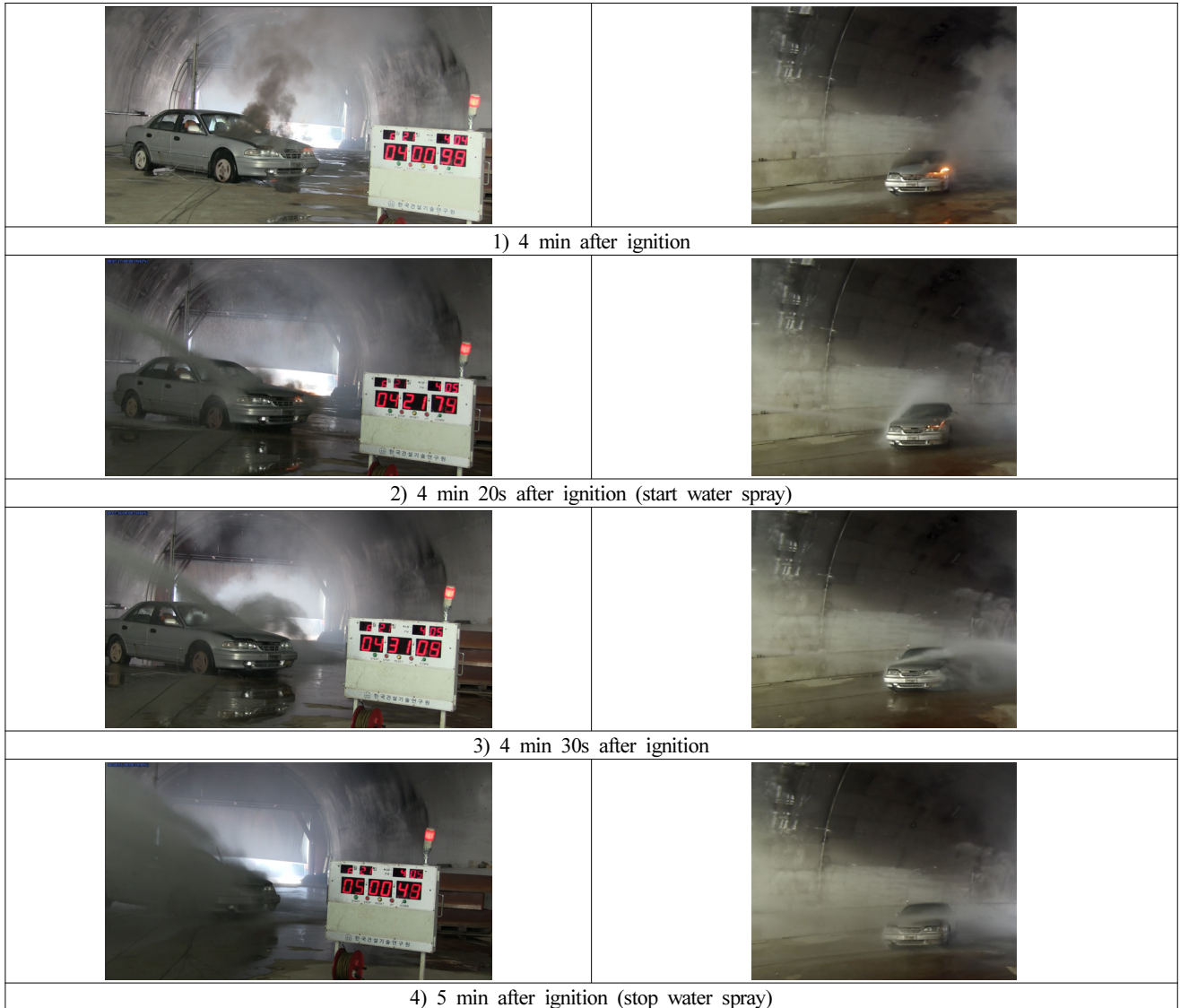
Figure 7. Result for case 2 (Engine room fire, Distance to fire source 10 m).
