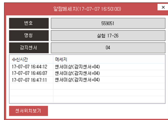
Fig. 18. Sensor alarm pop-up window when falling rock detection.
