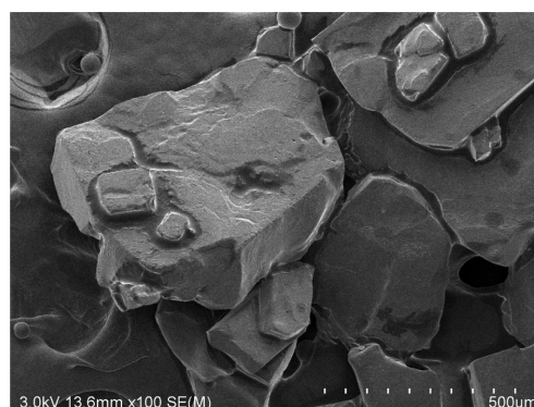
Fig. 2. SEM photograph of 1% crosslinked 1-aza-18-C-6-styrene-DVB resin.
