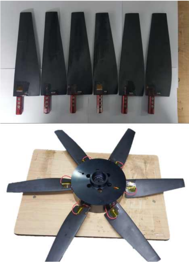
Fig. 7 Fabricated Blades and Installation on Hub
