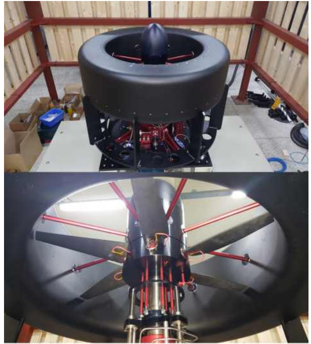
Fig. 8 The Assembly of Duct Fan Test Equipment
