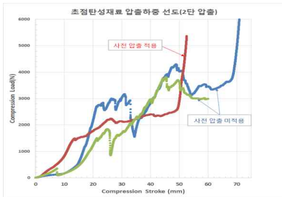
Fig. 17 Load-Stroke Curve(2 Stage Extrusion)
