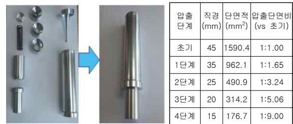
Fig. 15 Shock Absorber Components & Multi-Extrusion Ratio
