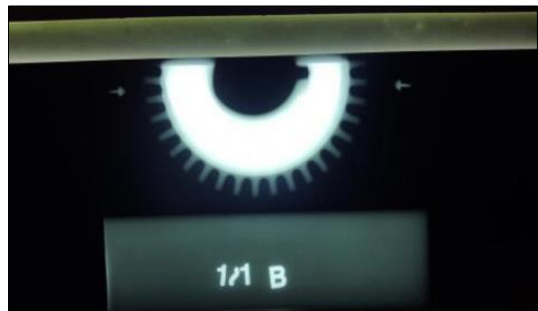
Fig. 18 Life Test 0% X-ray nondestructive inspection photo of Hub
