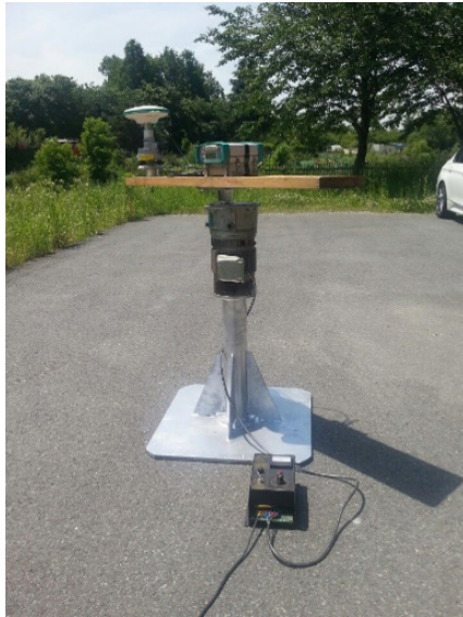
Fig. 3. Setup of a kinematic test using a turntable.
