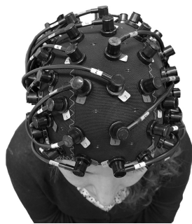
Figure 2. fNIRS head cap, developed by Hitachi
