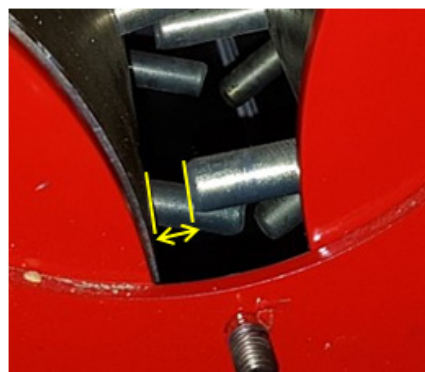
Figure 11. Radial clearance between rotating drum and cylindrical teeth.
