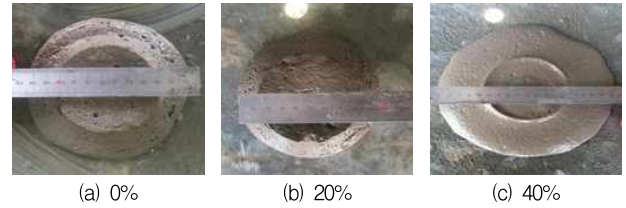
Figure 2. Flow images of aerated concrete specimens
