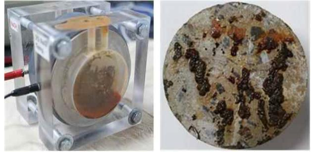
Figure 7. Corrosion during the chloride ion penetration resistance test of steel fiber reinforced concrete
