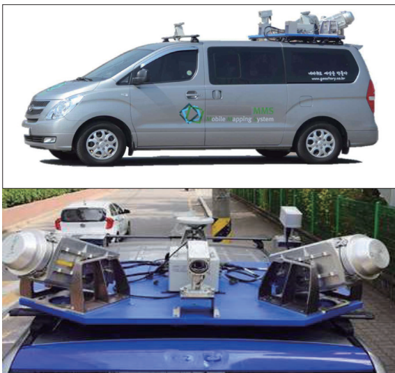
Fig. 2. Mobile mapping system (source: MOLIT, 2017)
