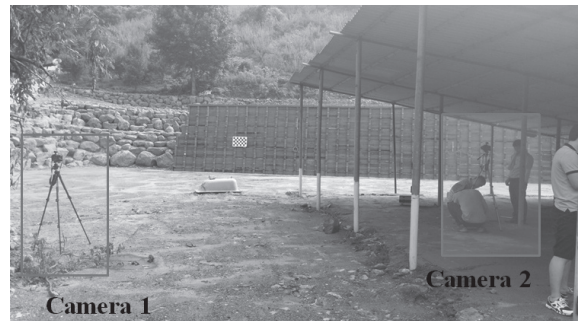
Fig. 5. Cameras set-up for photogrammetry
